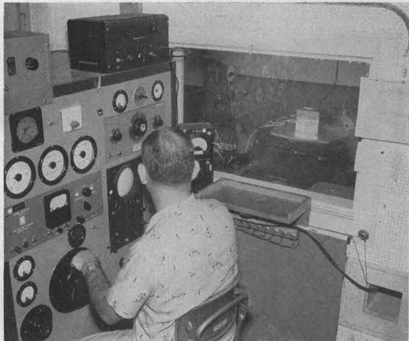
VIBRATION MISERIES — The howl of a shake table, seen through the window of a soundproof room, would greatly irritate operators if it were not safely enclosed as shown here. This is but one example of how the industrial hygienist makes working conditions more pleasant.
